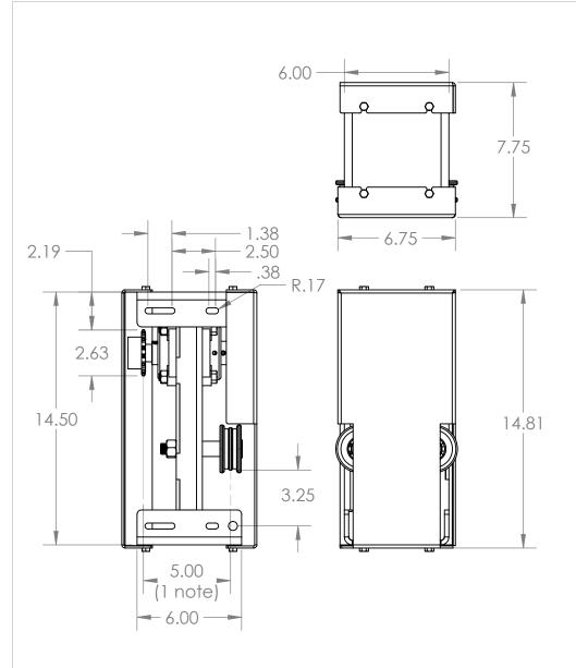
(1) could be field adjusted up to 7" for 4" thick gates
